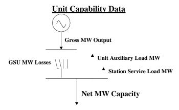
Net MW Capacity = (Gross MW Output - GSU MW Losses - Unit Auxiliary Load MW - Station Service Load MW)
